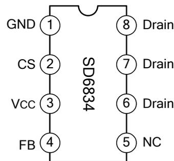
**Note:** it is recommended to connect pin 5 to pin Drain for better heat dissipation.
