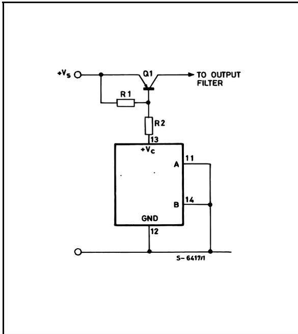
For single-ended supplies, the driver outputs are grounded. The  $V_c$  terminal is switched to ground by the totem-pole source transistors on alternate oscillator cycles.
