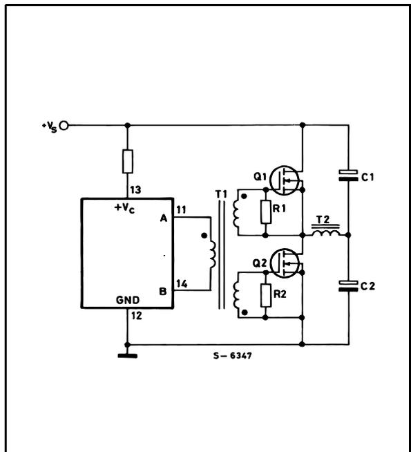
Low power transformers can be driven directly. Automatic reset occurs during dead time, when both ends of the primary winding are switched to ground.
