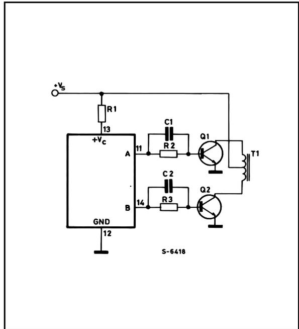
In conventional push-pull bipolar designs, forward base drive is controlled by  $R_1 - R_3$ . Rapid turn-off times for the power devices are achieved with speed-up capacitors  $C_1$  and  $C_2$ .
