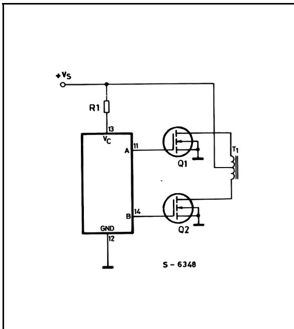
The low source impedance of the output drivers provides rapid charging of Power Mos input capacitance while minimizing external components.
