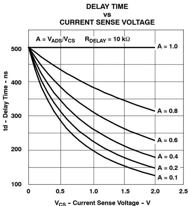
Figure 5. Delay Time Under Varying ADS Voltages
